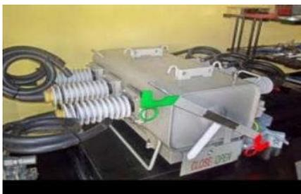
Gambar 2. Load Break Switch (LBS)
