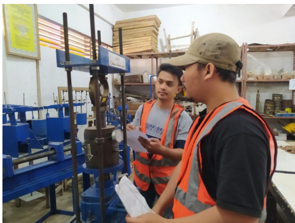
Gambar 2. Uji CBR laboratorium
