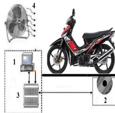
Gambar 1 Skema uji dynamometer ; (1) monitor, (2) roller dynamometer , (3) GPU ( graphic processing unit ), (4) kipas blower
