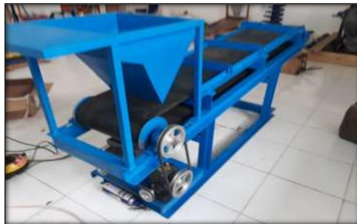
**Gambar 4.** Alat Magnetik Separator Skala Laboratorium
