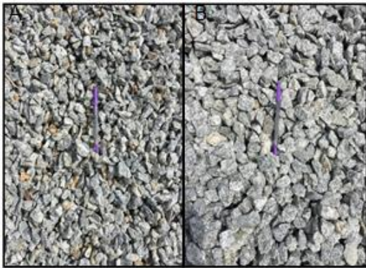
Gambar 9. Produk Akhir Secondary Crusher (a) Split 1–2, (b) Split 2–3
