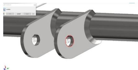
Gambar 7 Fixed Constraint
