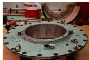
Gambar 5 Turbin Guide Bearing
