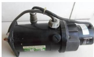
Gambar 4 Servo Motor
