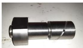
Gambar 3 Shear Pin
