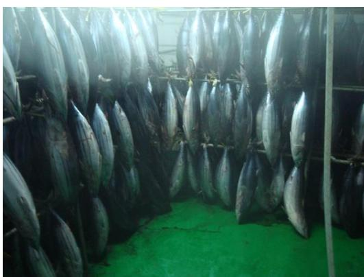
**Gambar 1 Air blast freezer tipe batch**
