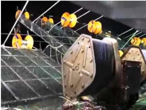
Gambar 1. Mesin Pancing Cumi-Cumi Otomatis
