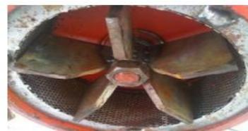
Gambar 1. *Hammer mill* (Purnomo, 2013)
