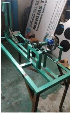
Gambar 5. Prototip PLTGL Sistem Linkage
